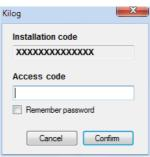
The access to the measurement correction is protected by a password associated to the installation key. To obtain this code, please contact KIMO.
